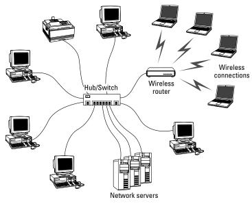
Figure I-1: Local area networks connect computing devices in close proximity.
